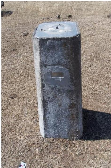
**Figure 30** NSW 1972 Trigonometry Survey Marker
