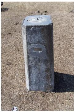
Figure 30 NSW 1972 Trigonometry Survey Marker
