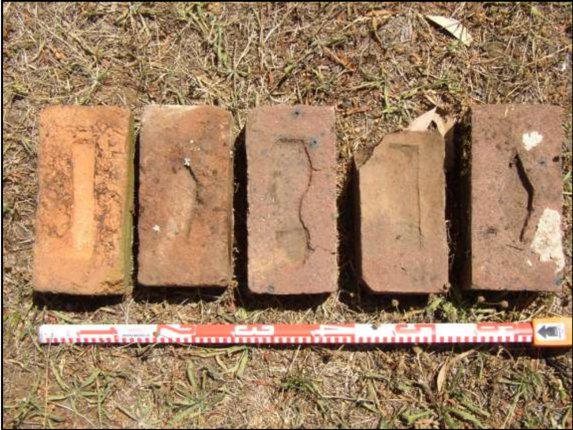
Plate 353: P9. Selection of bricks on the site showing different frogs.
