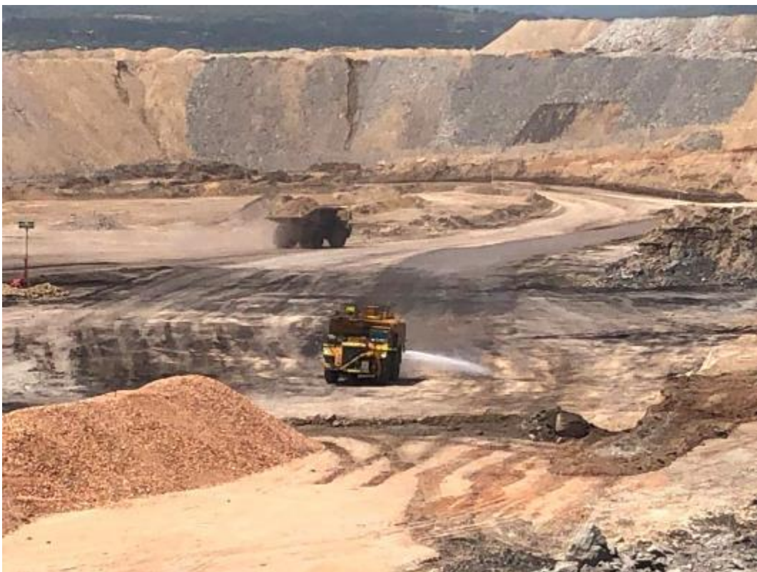
Photo Air 2 - Haul truck dust along haul route compared to area recently watered
