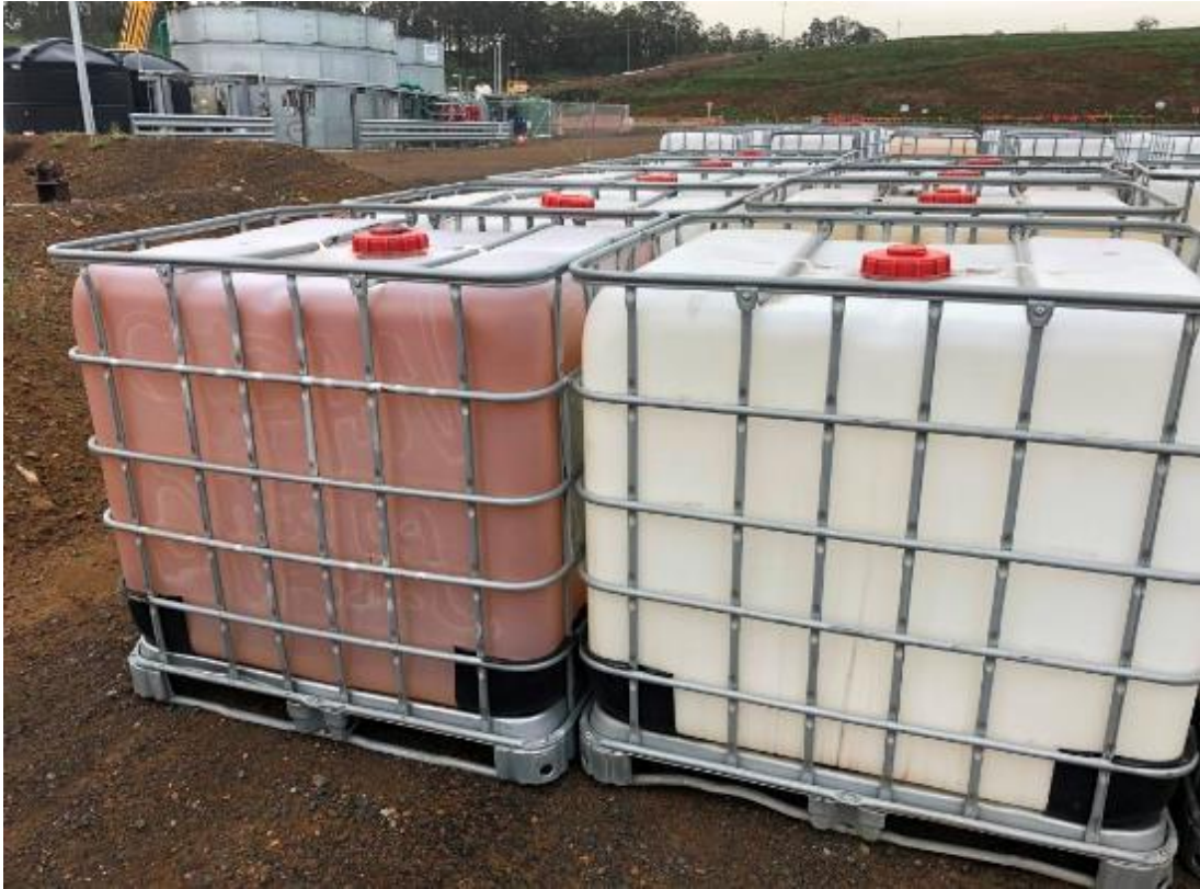
Waste Photo 5 - Workshop area - Bulky bins not stored in bunds
