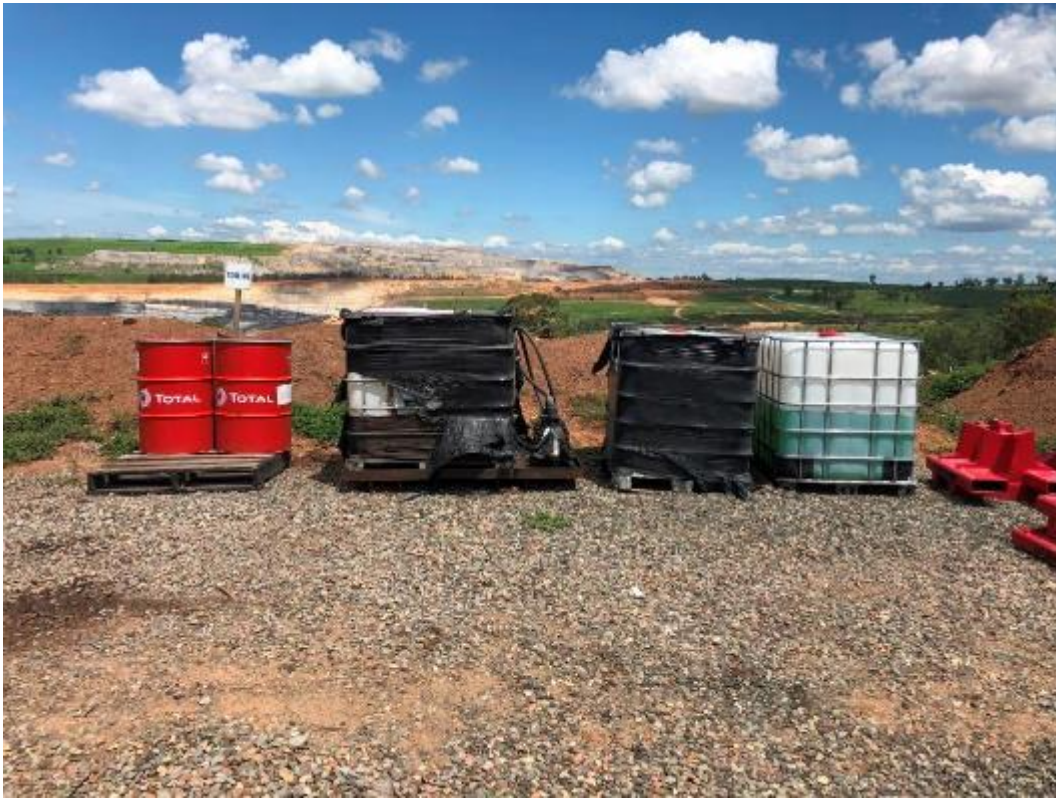
Waste Photo 1 - Inpit storage area containing unbanded containers and bulky bins
