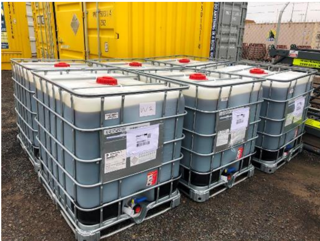
Waste Photo 4 - Workshop area - Gear oil not stored in bund
