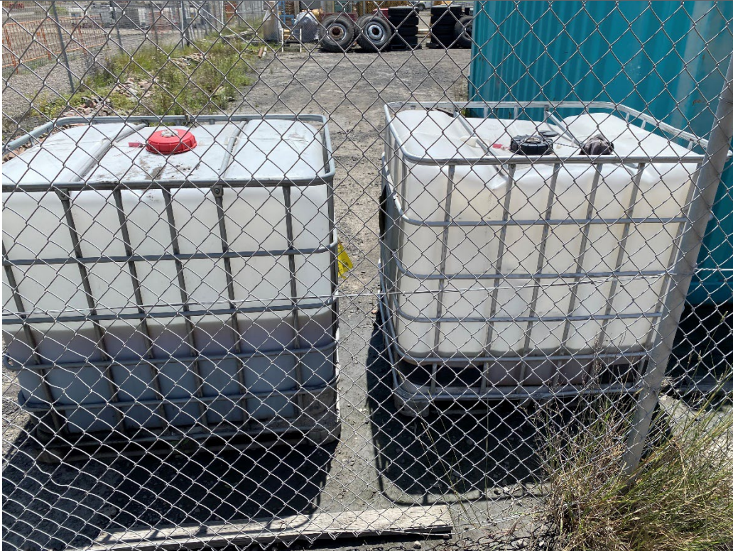
Plate 13 – Old workshop hydrocarbon cubes on unbanded pallets
